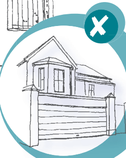
INAPPROPRIATE METAL FOLDING DOOR SET INTO BOUNDARY WALL WHICH DISREGARDS HISTORIC BOUNDARY WALLS, LACK OF SCALE, ETC.
